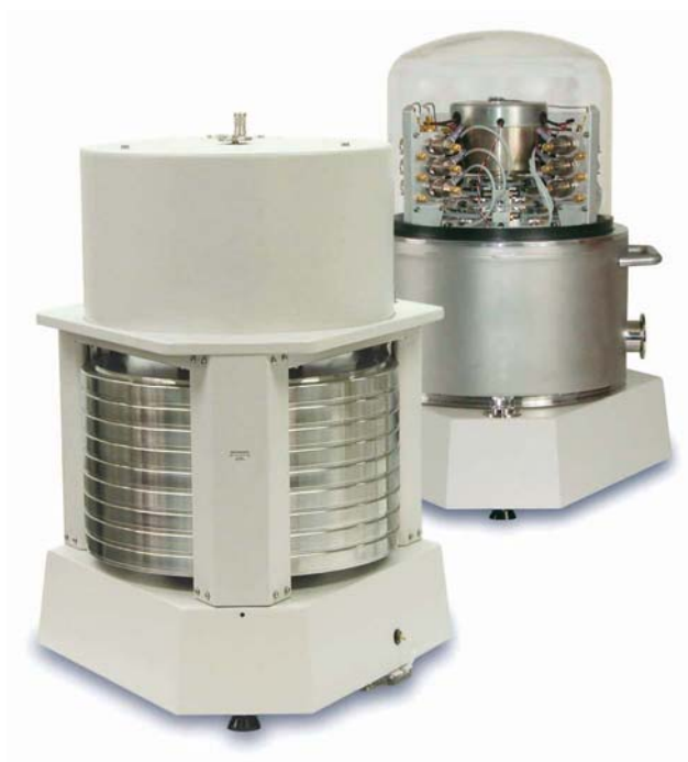
Figure 7. Automated mass handling systems on PG7000 pressure balance platforms, 100 kg (foreground) and 38 kg with vacuum reference versions.
