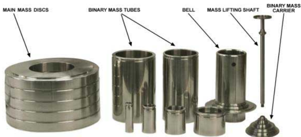
Figure 3. Complete mass set for automated mass handling system.
